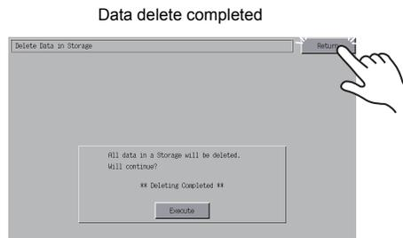
\* Data in storage is completely deleted. However, redisplaying the Main Menu screen by the [Return] switch will automatically create the access folder of the screen data transferred to MONITOUCH.
