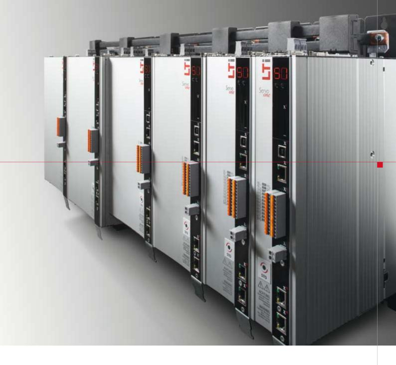
A cost-effective, space-saving variant for supply to the DC axis modules, with a low simultaneity factor, is provided via the DC link of a ServoOne single-axis (Shared-DC system). In this, the total power output of the DC link corresponds to the output of the AC axis module. Kinetic braking energy is converted into heat by way of a shared braking resistor.
